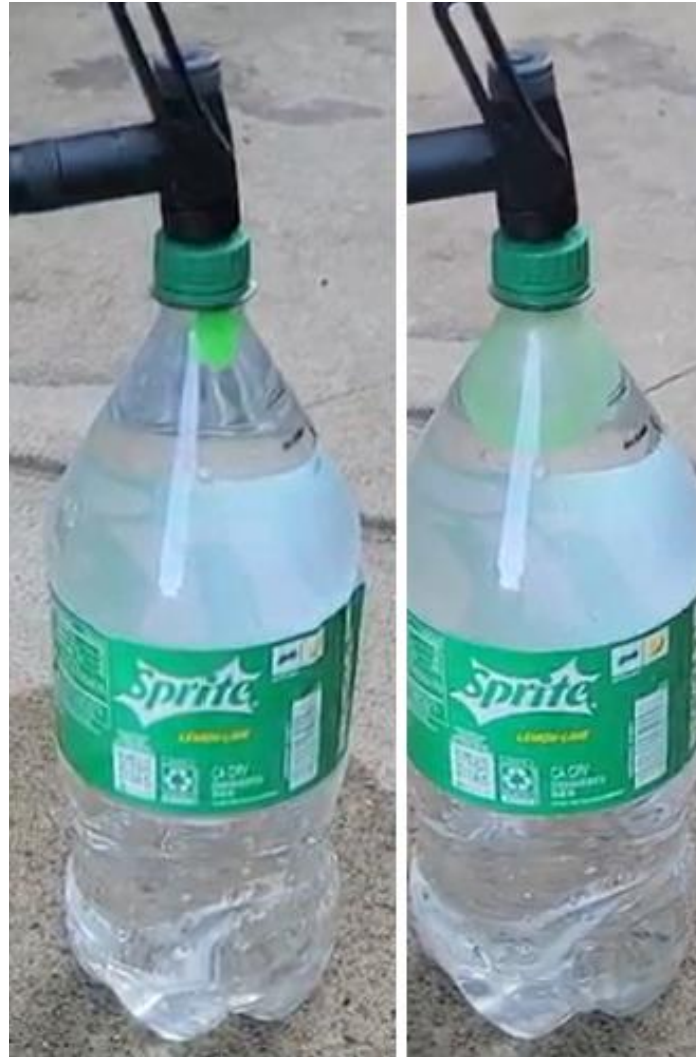
Prototype accumulator shown depressurized(left) and pressurized(right)
